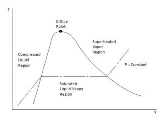
The liquid-vapor transition in a fluid
